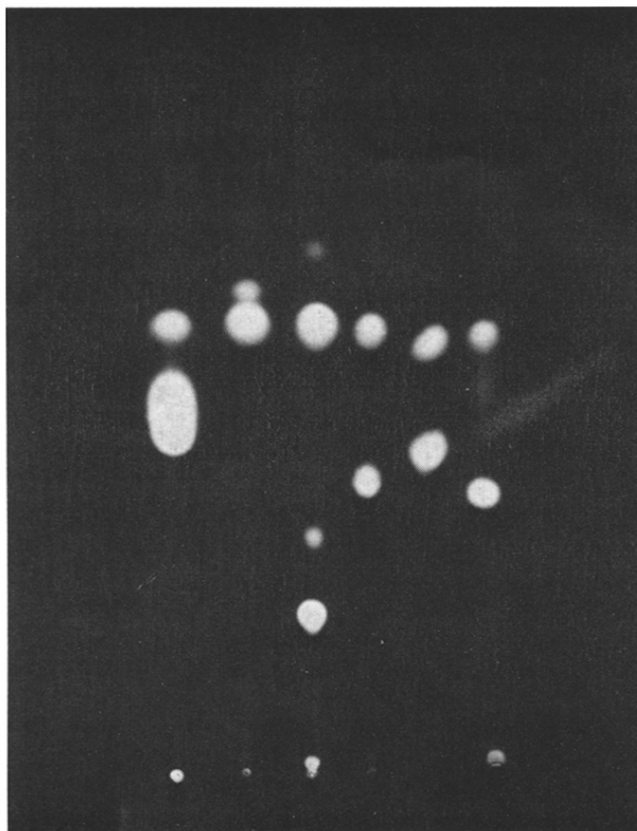
Fig. 1. TLC of Dns compounds on a sheet of Polyamide A 1700. From left to right: Dns-adenine, -cytosine, -guanine, -thymine, -uracil and -xanthine. The solvent was 6% HCOOH. The spot in common to each lane is hydrolyzed reagent (Dns-OH), a side-product always present in Dns derivatized samples.
